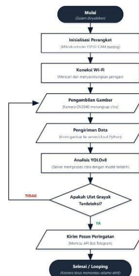
Gambar 2. Flowchart sistem deteksi ulat grayak
